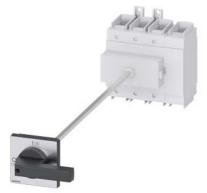
SENTRON, Switch disconnector 3LD, main switch, 4-pole, lu: 160 A, Operating power / at AC-23 A at 400 V: 75 kW, floor mounting with door coupling, knob-operated mechanism, black, 4-hole mounting of the handle
