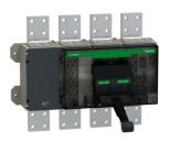
Circuit breaker frame, ComPacT NS2500N, 50kA at 415VAC, 2500A, 4P, fixed, manually operated, without control unit
