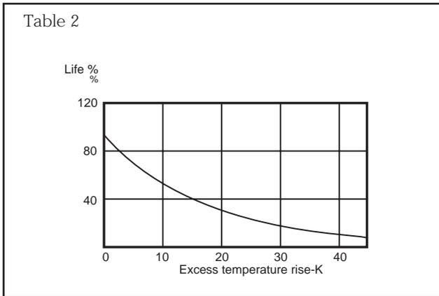
The graph illustrates the effect of exceeding the highest permitted winding temperature on winding life.
