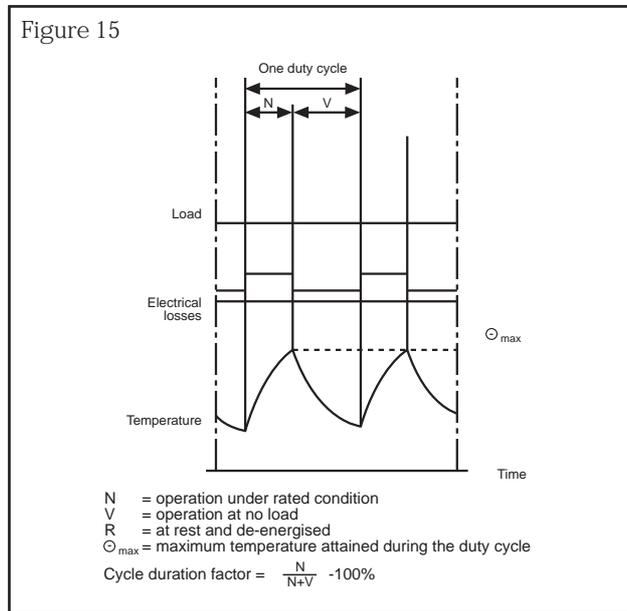
**S7 continuous operation, periodic duty with electrical braking**
