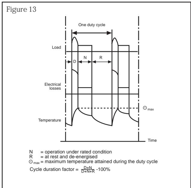
**S5 intermittent duty with electrical braking**
