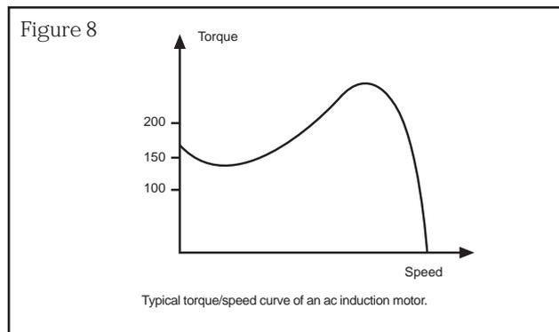
Typical torque/speed curve of an ac induction motor.
