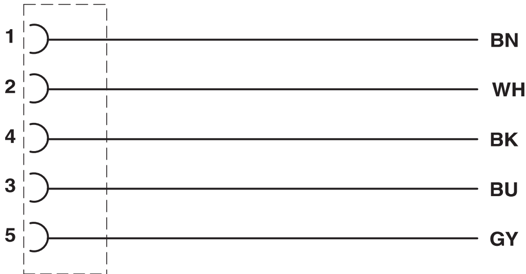
Contact assignment of the M12 socket
