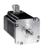
3-phase stepper motor - 13.5 Nm - shaft Ø19 mm - L=180 mm - with brake- term box
