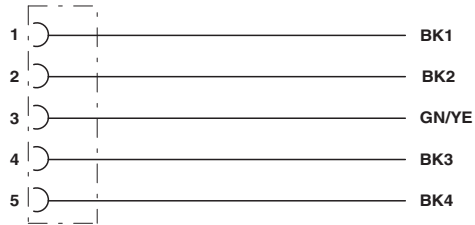
Contact assignment of 7/8" socket
