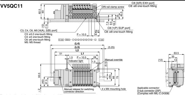
The dashed lines indicate the DIN rail mounting [-D] (with DIN rail mounting bracket)
