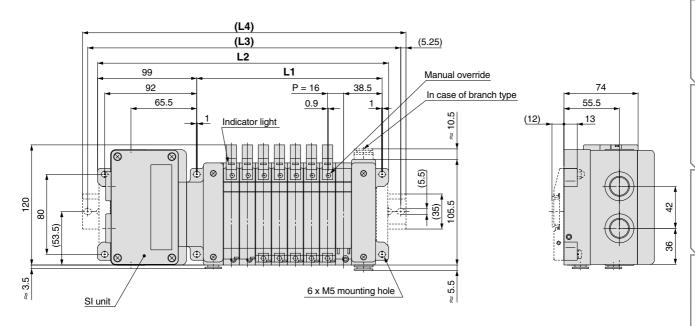
The dashed lines indicate DIN rail mounting [-D] (with DIN rail mounting bracket).
