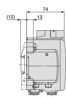
The dashed lines indicate DIN rail mounting [-D] (with DIN rail mounting bracket).
