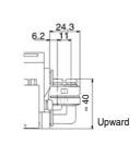
DIN rail mounting bracket [-D] VVQ1000-57A {For F/L/M/P/S (EX500) kit} VVQC1000-57A-S {For S (EX250) kit} VVQC1000-57A-T (For T kit)
