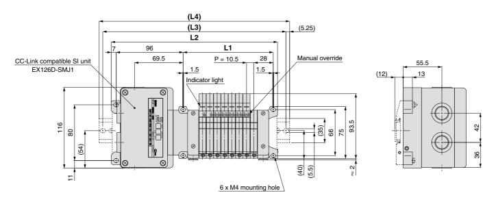
The dashed lines indicate DIN rail mounting [-D] (with DIN rail mounting bracket).
