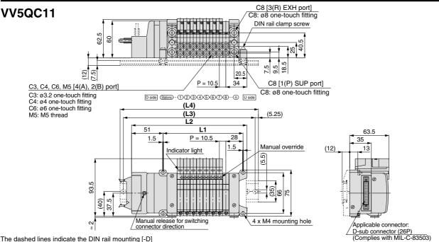
The dashed lines indicate the DIN rail mounting [-D] (with DIN rail mounting bracket)
