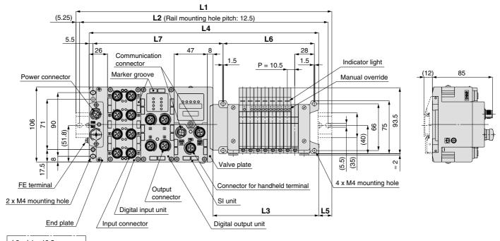
L2 = L1 - 10.5L3 = 10.5 x n1 + 65.5  $L4 = L3 + 81 + 47 \times n2$ L5 = (L1 - L4)/2 $L6 = 10.5 \times n1 + 45$  $L7 = 47 \times n2 + 89.8$
