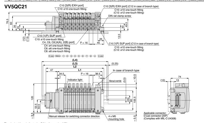
The dashed lines indicate the DIN rail mounting [-D] (with DIN rail mounting bracket).
