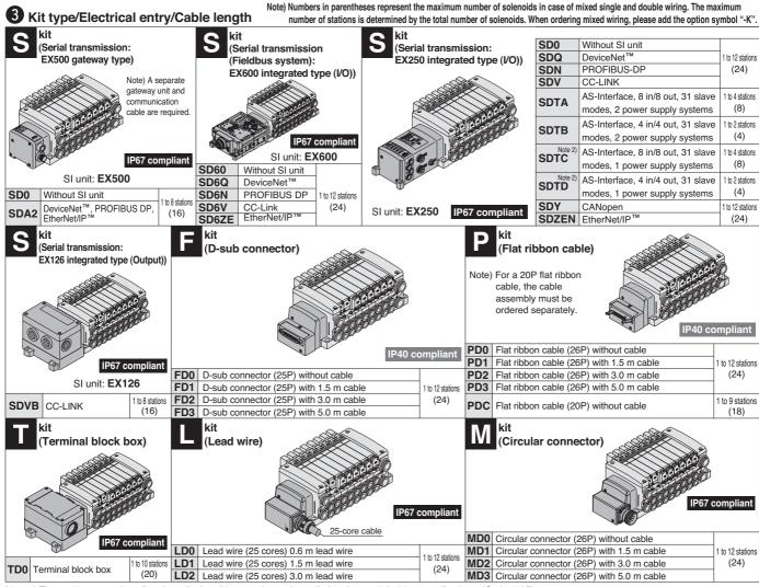
Note 1) The maximum number of stations displayed in parentheses is applied to the special wiring specifications. (Option "-K")
