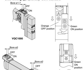
The manual override is locked by sliding it all the way to the pilot valve side (ON side) with a small flat head screwdriver or with your fingers. Slide it to the fitting side (OFF side) to release it. In addition, it can also be used as a push type by using a screwdriver, etc., of ø1.7 or less. (ø2 or
