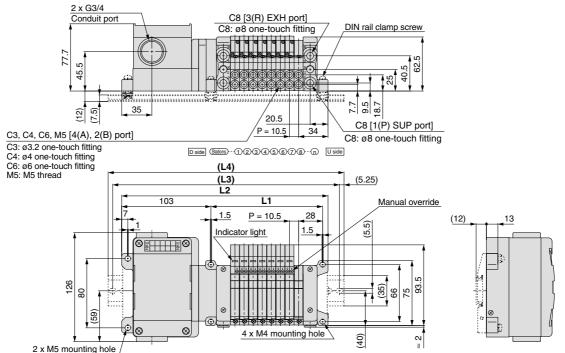
The dashed lines indicate DIN rail mounting [-D] (with DIN rail mounting bracket)
