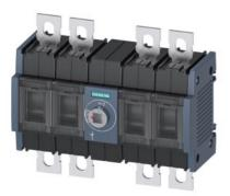
Switch disconnector 80 A, Size 2, 4-pole Front operating mechanism center Basic unit without handle flat terminal incl. phase barriers
