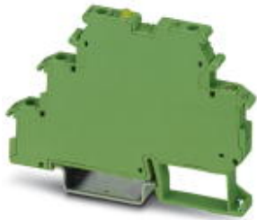
Power solid-state relay terminal block, input: 24 V DC, output: 3 - 30 V DC/3 A, terminal block width: 6.2 mm
