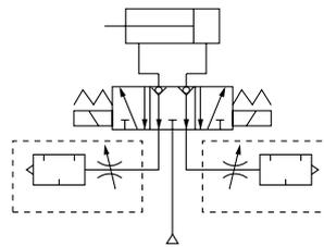
Residual pressure behind the exhaust needle may cause check valve malfunction in the "Perfect Valve".
