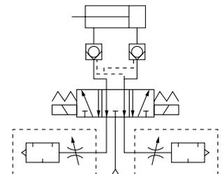
Residual pressure behind the exhaust needle may cause check valve to malfunction.
