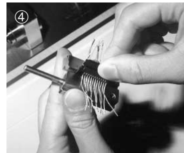
6. Pull down the handle. The wiring and cutting of excess cable length are completed.
