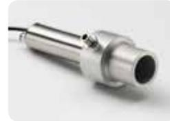
The air purge collar is used to keep dust, fumes, moisture and other contaminants away from the lens. Air flows into the fitting on the side and out of the aperture at the front.
