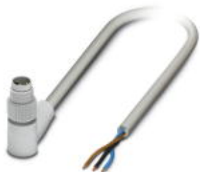
Sensor/Actuator cable, 3-position, PP-EPDM halogen-free, Gray RAL 7035, Plug angled M8, on free cable end, Cable length: 10 m, Hygienic design, with plastic knurl
