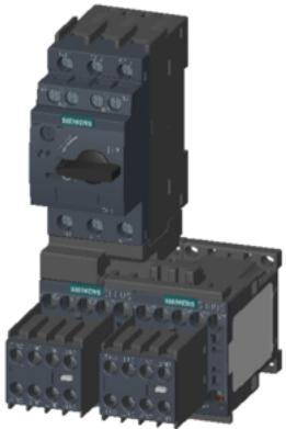
Load feeder fuseless, Reversing duty 400 V AC, Size S00 1.4...2 A 24 V DC screw terminal for installation on standard mounting rail (also fulfills type of coordination 1) Type of coordination 2,  $I_q = 150 \text{ kA}$  1 NC (contactor) 1 NO+1 NC (circuit breaker, transverse)
