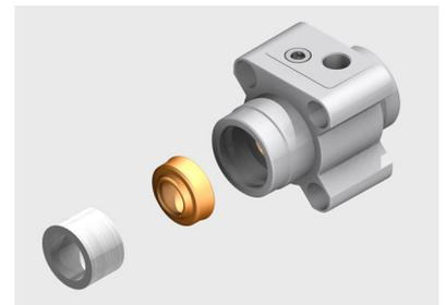
15. Push together the circlip (e.g. with the help of pliers) and insert into the bearing cap.
