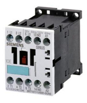
CONTACTOR, AC-3 4 KW/400 V, 1 NO, DC 24 V, 3-POLE, SIZE S00, SCREW CONNECTION
