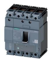
circuit breaker 3VA1 IEC frame 160 breaking capacity class S Icu=36kA @ 415V 4-pole, line protection TM220, ATFM, In=63A overload protection Ir=44A...63A short-circuit protection Ii=10 x In N conductor unprotected nut keeper kit
