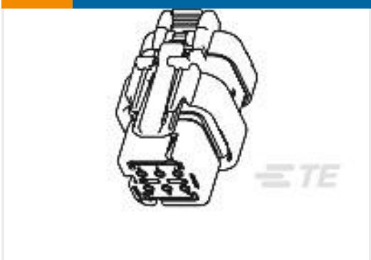
TE Part #776494-2 AS 16, 8P PLUG ASSY, KEY 2
