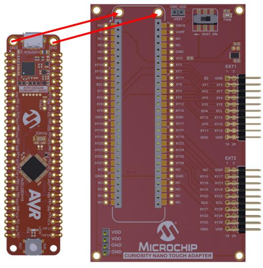
Figure 5-1. Curiosity Nano Touch Adapter Mounting
