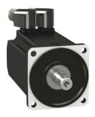
servo motor BMH, Lexium 32, 3.3Nm, 6000rpm, keyed shaft, with brake, IP54, 16 multiturn encoder
