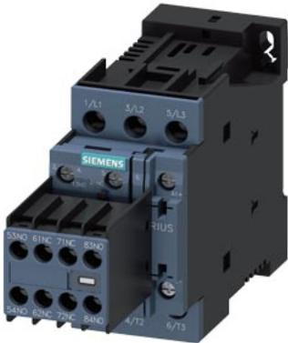
power contactor, AC-3e/AC-3, 25 A, 11 kW / 400 V, 3-pole, 24 V DC, with plugged-in diode combination, auxiliary contacts: 3 NO + 3 NC, screw terminal, size: S0, with 3RH2911-1XA22-0MA0
