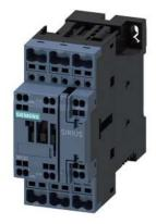
power contactor, AC-3e/AC-3, 17 A, 7.5 kW / 400 V, 3-pole, 24 V DC, with plugged-in diode combination, auxiliary contacts: 1 NO + 1 NC, spring-loaded terminal, size: S0
