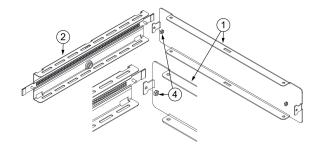
Assemble Side Frame to Front Rear Panel with 4xNut M3.
