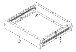
2. Complete Side Frames and Front Rear Panel assembled.
