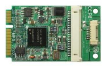
Taiwan Commate Computer Inc. (COMMELL), announced its new USB 3.0 Super-Speed PCI Express mini card -- MPX-7202, the Super-Speed USB 3.0 is the next revolution in I/O interconnect standards that will works up to 5 Gbps data transfer when connecting to USB 3.0 compliant peripherals, with 10 times faster throughput than USB 2.0 standard, and maintaining compatibility with existing USB 2.0 or USB 1.1 peripheral devices.
