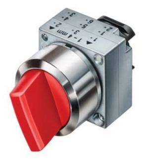
22MM METAL ROUND ACTUATOR: SELECTOR SWITCH MOMENTARY CONTACT TYPE 3 SWITCH POSITIONS I-O -II NON-ILLUMINATED WITH HOLDER RED
