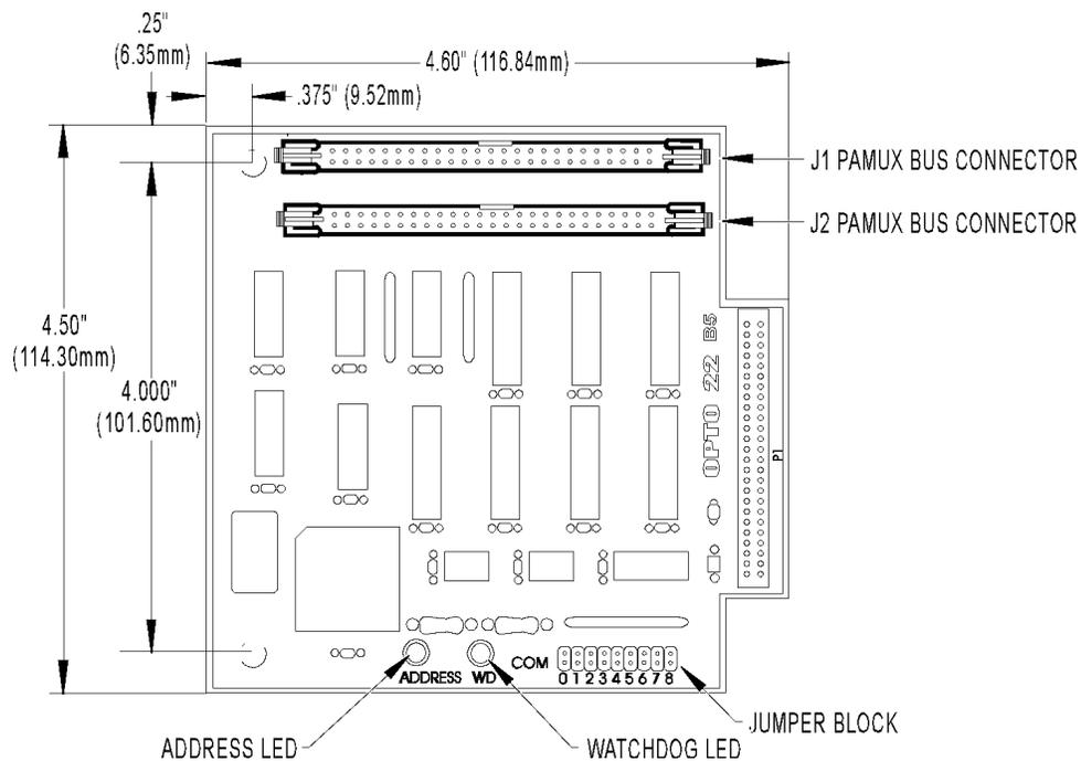
Figure 2: Dimensions of the B5 Brain Board
