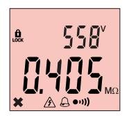
On the other hand, if the measurement is below the threshold, the instrument emits a continuous beep, the backlighting lights red, and the \*\*symbol is displayed.
