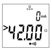
If the display unit indicates  $>42.00\Omega$ , the fuse has blown and must be replaced.
