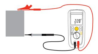
The instrument displays the AC+DC voltage. If it is >30V, the 🖄 symbol is displayed to warn the user that the voltage on the terminals is hazardous.
