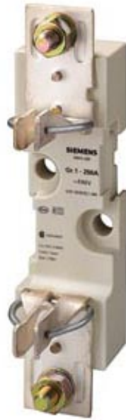
LV HRC FUSE BASE 690V(1000V) SINGLE-POLE, 250A, SIZE 1 PAD-TYPE TERMINAL
