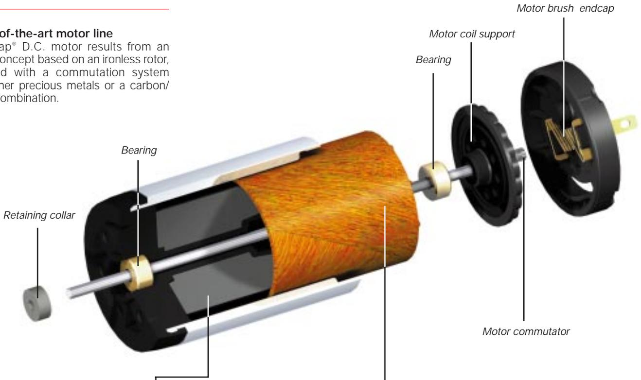
The stator part consists of a cylindrical two-pole permanent magnet, placed inside a steel tube closing the magnetic circuit. High quality rare earth or AlNiCo magnets ensure very high performance in a small envelope.
