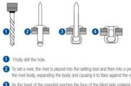
2 To set a rivet, the rivet is placed into the setting tool and then into a pre-drilled hole. It is fixed by the jaws within the tool pulling the mandrel head into the rivet body, expanding the body and causing it to flare against the reverse (blind) side of the application.
