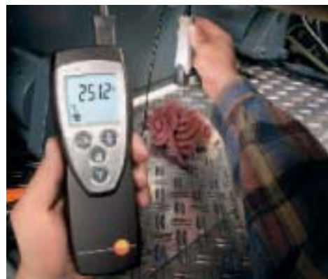
Temperature measurement in semi-solid materials with the superfast penetration probe, ideal for plastics, foodstuffs etc.
