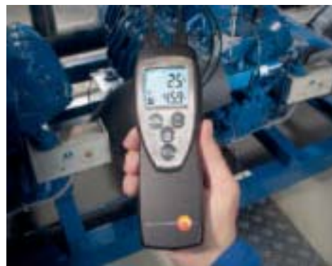
Simultaneous measurement of overheating and undercooling in refrigeration systems with testo 922
