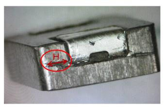
Figure 1: Hairline crack and definition of H
