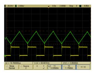
Figure 13: Inductor current and switching
