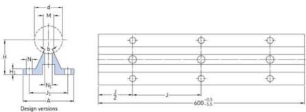
Design versions LRCB = Shaft support with mounting holes LRCC = Shaft support without mounting holes
