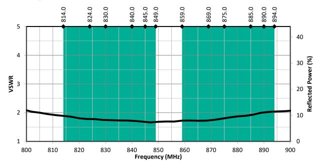
Figure 1. PW LTE Band 5 Antenna VSWR with Band 5 Uplink/Downlink Highlights
