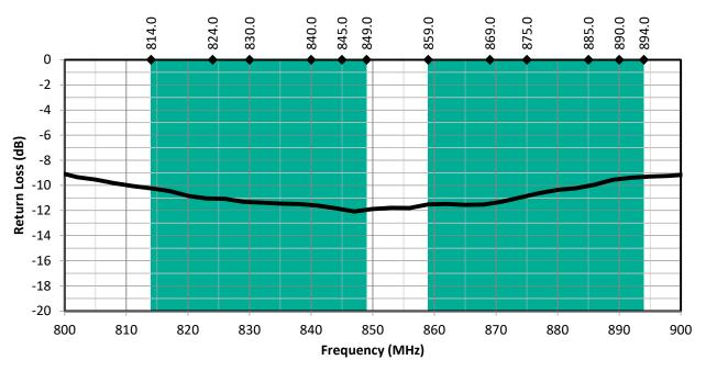
Figure 2. PW LTE Band 5 Antenna Return Loss with Band 5 Uplink/Downlink Highlights
