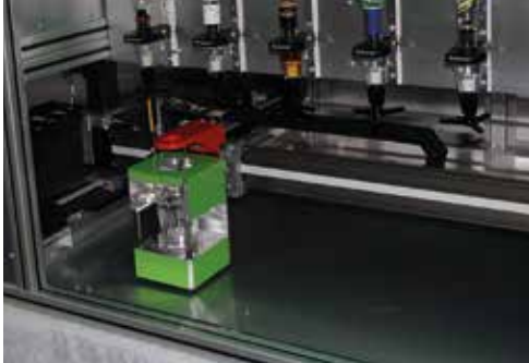
The lubrication-free, easy-to-clean guide system is in the form of a drylin® standard multi-axis room linear robot DLE-RG-001
