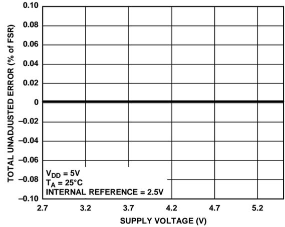
Figure 29. TUE vs. Supply, Gain = 1
