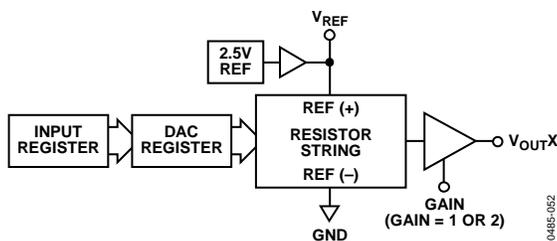
Figure 48. Single DAC Channel Architecture Block Diagram
