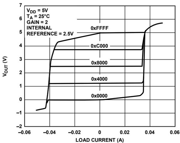
Figure 34. Source and Sink Capability at 5V
