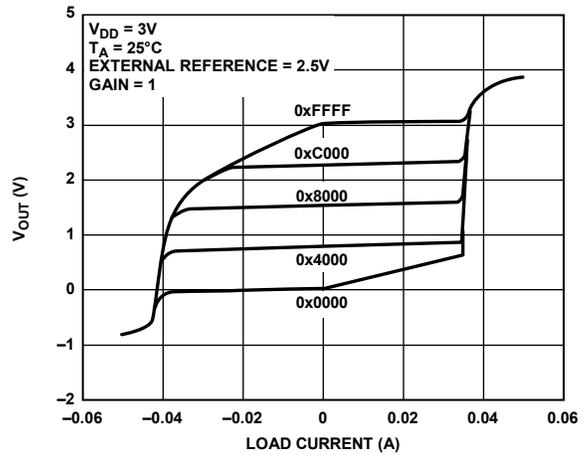
Figure 35. Source and Sink Capability at 3V
