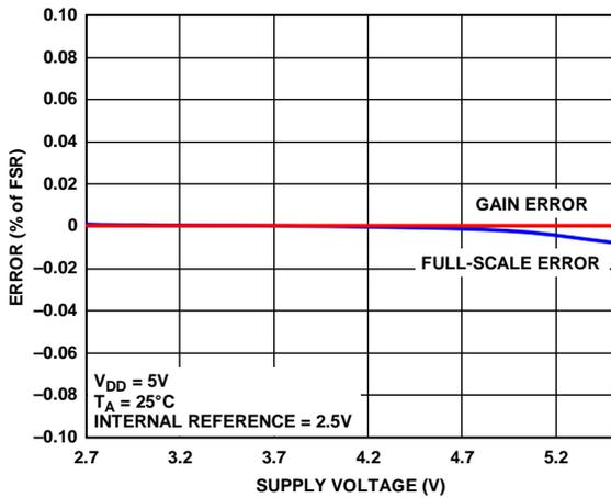
Figure 26. Gain Error and Full-Scale Error vs. Supply
