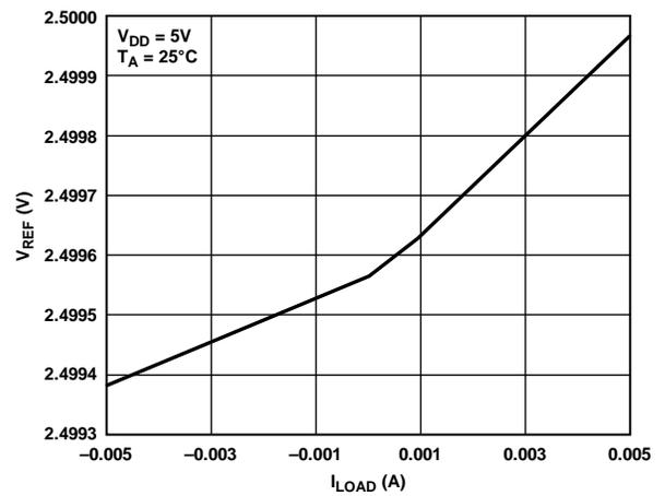
Figure 13. Internal Reference Voltage vs. Load Current
