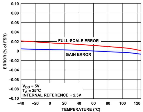
Figure 24. Gain Error and Full-Scale Error vs. Temperature
