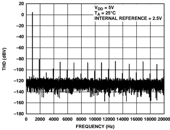
Figure 45. Total Harmonic Distortion at 1 kHz
