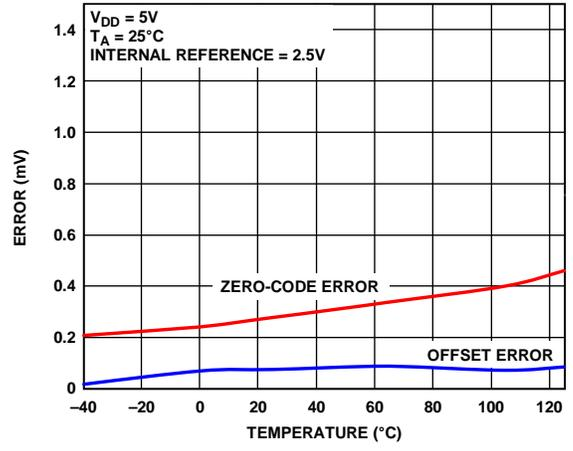
Figure 25. Zero-Code Error and Offset Error vs. Temperature
