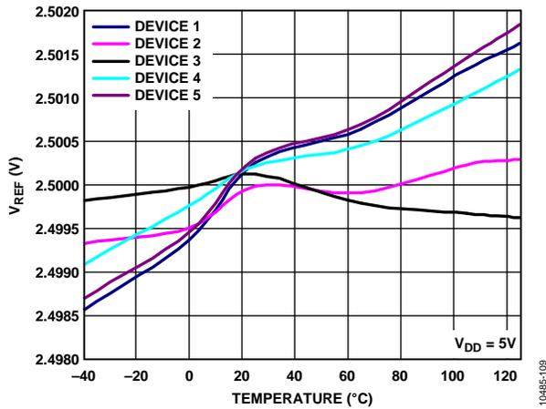
Figure 9. Internal Reference Voltage vs. Temperature (Grade A)
