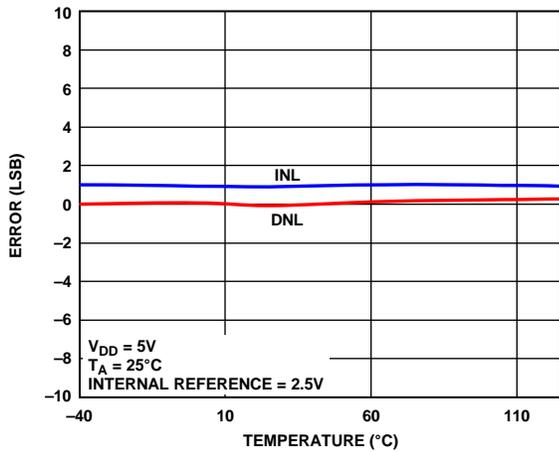
Figure 21. INL Error and DNL Error vs. Temperature
