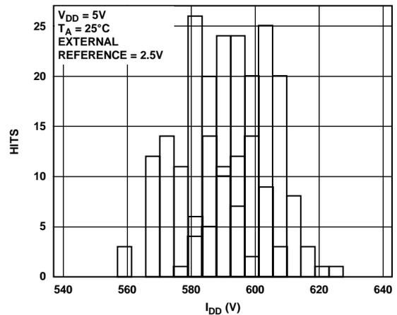
Figure 31.  $I_{DD}$  Histogram with External Reference, 5 V
