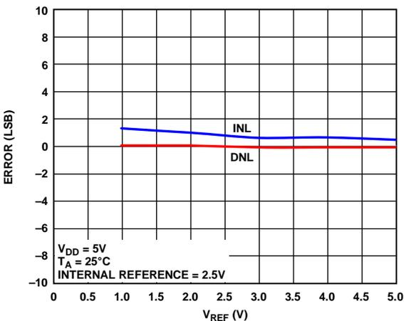
Figure 22. INL Error and DNL Error vs.  $V_{REF}$
