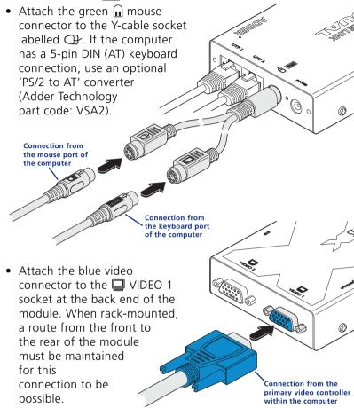
3 At the other end of the KVM cable, attach the keyboard, mouse and video connectors to the appropriate sockets at the rear of the computer system. Note: For computers equipped with two video controllers, the video connector on the KVM cable should go to the output socket of the primary controller.
