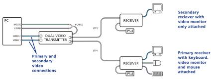
In this mode, the primary and secondary remote receiver modules are connected differently. For the primary receiver, use the connection details shown on the previous page. For the secondary receiver, connect the module as shown here:
