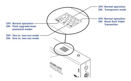
Note: When shipped, all switches are set in the OFF positions and this will produce normal operation in the 'Two-in, two-out' mode. To select the alternative, 'One-in, two-out' mode, simply change switch 3 to the ON position.
