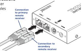
Note: In the 'Two-in, two-out' mode, the UTP 1 connector provides keyboard, video and mouse data, while the UTP 2 connector supplies only a secondary video signal.
