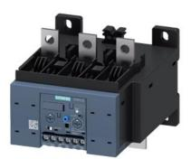
Overload relay 50...200 A for motor protection Size S6, CLASS 5...30E Contactor mounting/stand-alone installation Main circuit: busbar connection Auxiliary circuit: Screw terminal Manual-Automatic-Reset Internal ground fault detection
