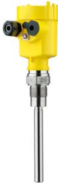
Due to the advantageous rod shape, jamming, e.g. caused by granules, is impossible. Since installation position and granule size do not influence the sensor, adjustment with medium is not necessary. The VEGAVIB vibrating rod operates at a frequency of approximately 350 Hz.
