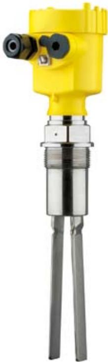
VEGAWAVE switches are extremely robust. The piezo drive is screwed together to make it as reliable as possible. This tuning fork measures limits in practically any bulk solid application. It operates at a frequency of approximately 200 Hz. Adjustment with medium is not required.
