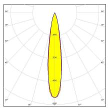
Dimensions: 50.0 mm x 50.0 mm Height: 10.70 mm ~15° spot beam with 6 optics
