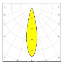
Dimensions: 50.0 mm x 50.0 mm Height: 10.70 mm ~20° medium beam with 7 optics
