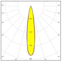
Dimensions: 50.0 mm x 50.0 mm Height: 10.70 mm ~15° spot beam with 4 optics
