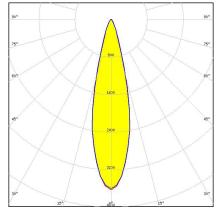
Dimensions: 50.0 mm x 50.0 mm Height: 10.70 mm ~20° medium beam with 5 optics
