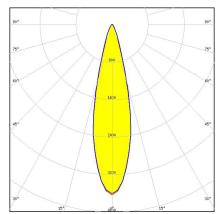
Dimensions: 50.0 mm x 50.0 mm Height: 10.70 mm ~20° medium beam with 6 optics
