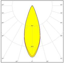
Dimensions: 50.0 mm x 50.0 mm Height: 10.70 mm ~30° wide beam with 5 optics
