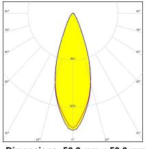
Dimensions: 50.0 mm x 50.0 mm Height: 10.70 mm ~30° wide beam with 3 optics
