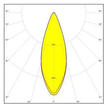
Dimensions: 50.0 mm x 50.0 mm Height: 10.70 mm ~30° wide beam with 6 optics
