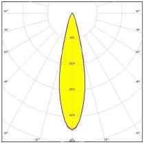
Dimensions: 50.0 mm x 50.0 mm Height: 10.70 mm ~20° medium beam with 3 optics
