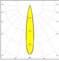
Dimensions: 50.0 mm x 50.0 mm Height: 10.70 mm ~15° spot beam with 3 optics
