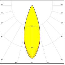
Dimensions: 50.0 mm x 50.0 mm Height: 10.70 mm ~30° wide beam with 4 optics
