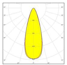
Dimensions: 50.0 mm x 50.0 mm Height: 10.70 mm ~30° wide beam with 7 optics
