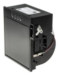
This RS Pro panel mount printer features a Seiko brand fixed head thermal line printer mechanism with a guillotine auto-cutter and anti-blockage design. It also has a large paper capacity. It has an electrical rating of 24VDC/2A and an RS232 + USB Interface.
