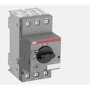
ABB's MS116 manual motor starters are electromechanical protection devices for the main circuit. They are mainly used to provide fuseless protection of motors against short-circuits, overloads and phase failures. In addition, they are used to switch motors ON/OFF manually. Starter combinations are setup together with contactors.
