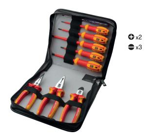
RS Pro 9 Piece VDE approved insulated pliers and screwdriver set with single pole voltmeter. Supplied in a vinyl wallet for secure transport and storage. The cutters, pliers and screwdrivers are ideal for working up to 1000 V AC or 1500 V DC. Suitable for cutting soft and hard wire.
