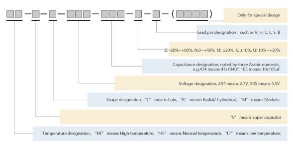
HESC5R5105Z-L means coin super capacitor 5.5V 1F V at normal temperature
