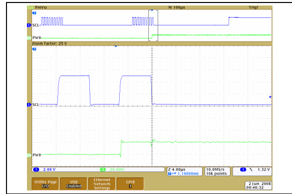
FIGURE 2-65: 100 k \Omega – Low-Voltage Increment Wiper Settling Time ( V_{DD} = 2.7\text{V} ) (1 \mu\text{s}/\text{Div} ).
