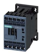
Contactor relay for railway 4 NO DC 24-34V, 0,7...1,25\*US, with integrated varistor Size S00, Spring-type terminal suitable for PLC outputs
