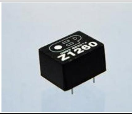
Provides isolation between modems or similar devices and telephone lines. This transformer is designed for use in voice or data transmission circuits where the line d.c. is diverted from the windings by a choke or solid state device. The use of this transformer should enable the equipment it is used with to comply with the relevant requirements of BS6305. This is a lower profile version of the OEP 1200 transformer.
