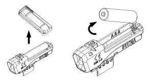
4. Ensure the battery cover is aligned properly on the LED flashlight. Reverse the sliding direction to close the battery cover.
