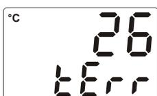
6- In programming section, when Tune operation is selected *YES*, if warning which is shown on the left blinks in operation screen for 10 seconds, it means that start conditions is not okay for Tune operation.
