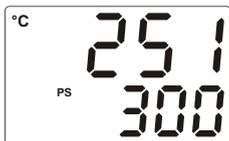
3- If value that is read from the analog input is higher than process set high limit parameter value  $P_{uPL}$ , value on the top display starts to blink like on the picture.
