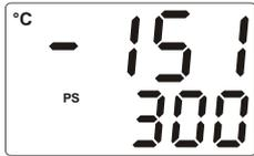
2- If value that is read from the analog input is lower than process set low limit parameter  $P_{LoL}$ , value on the top display starts to blink like on the picture.
