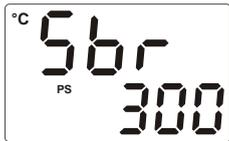
1- Sensor failure in analog inputs. Sensor connection is wrong or there is no sensor connection.
