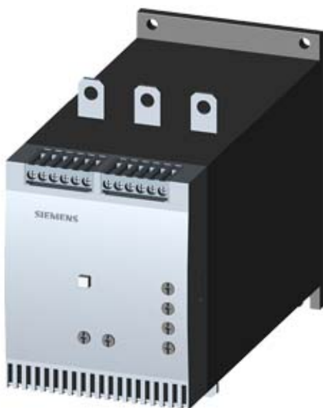
SIRIUS SOFT STARTER, S6, 134 A, 75 KW/400 V, 40 DEG., 200-460 V AC, 230 V AC, SCREW TERMINALS
